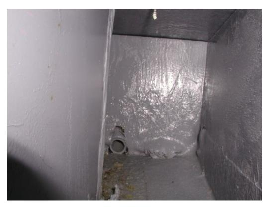
The fourth photo was taken near the preceding photo, but outboard of the stringer. Here the cutout is the evident, approximately half the height of the stringer at midships. Another Opti bag, and gear stored in the port locker.
