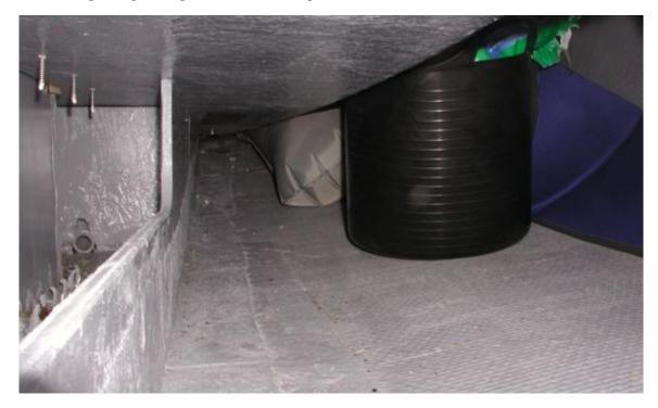
The next two photos are taken through the deck plate, under the teak bench in the aft bulkhead of the cockpit. The first is facing aft towards the transom. You can see the starboard cockpit drain to the left, and the bronze through hull to the right.
