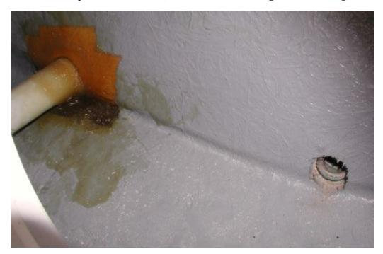
The last photo is facing forward, and we see the aft end of the stringer box, with a short transverse stringer glassed in place and the drain leading forward. Note also that it appears that the stringer box is filled with foam, further sealing the stringers to the hull, and providing some floatation. When I look back at the third photo, of the second transverse stringer, I believe I can see foam around the drain pipe there as well.
